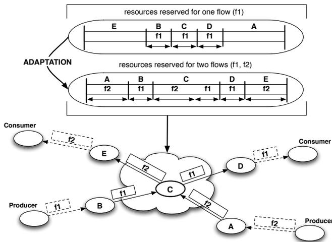
Figure 1: Adaptation example: the frame as perceived by  $C$ , is adapted to allocate resources for a new data flow ( $f_2$ ), preserving slots already assigned to another data flow ( $f_1$ ).
